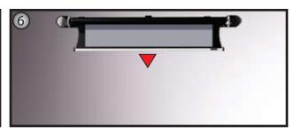
Deploy the screen and check your settings. The screen location will be higher then the original position.
