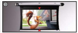
With the screen in the corrected position switch the screen motor power off. Reattach front valance to the Cabaret unit, ref manual image; #31-33 and you are done.
