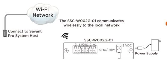
**HELPFUL!** No Ethernet connection is needed. The controller communicates with the Savant Pro System Host over the local Wi-Fi network.
