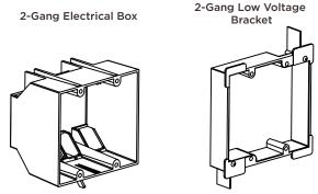
NOTE: If the Touch Panel is going to be installed with a Portrait orientation, the electrical box or bracket will need to be rotated
