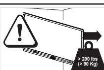
Do not move or mount the interactive flat panel by connecting rope or wire to its handles. Because the interactive flat panel is heavy, rope, wire or handle failure could lead to personal injury.
